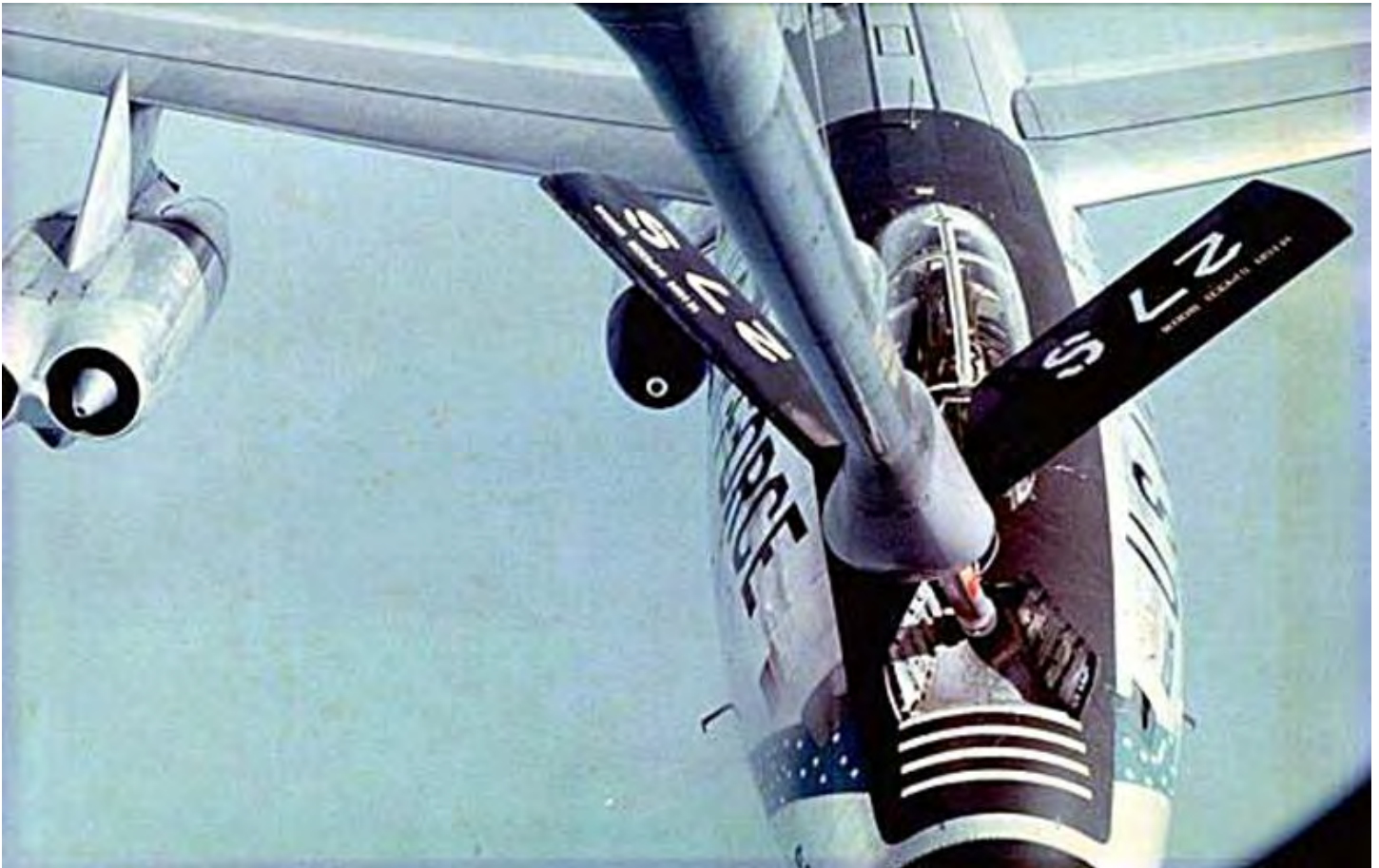
View of an RB-47 being refueled in flight.
