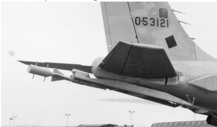
Because of the frequency of the targeted Hen House radar (155-165MHZ), reflection from the aircraft could impact the accuracy of the collected data if the antenna was mounted on the aircraft skin, and thus, isolation from any reflected energy had to be insured. While flying in other than sensitive areas of interest, the antenna was kept in the stowed and locked position.
