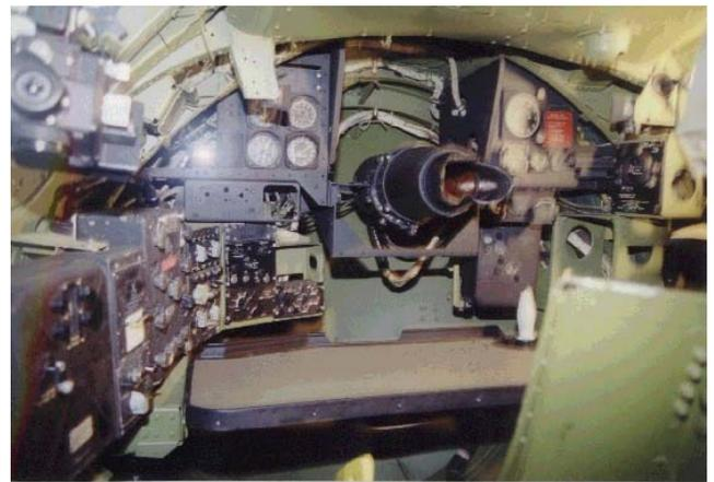
*Navigator's station in the nose. Restoration could not find a ten-inch radarscope, so they likely got this one from a tanker.*
